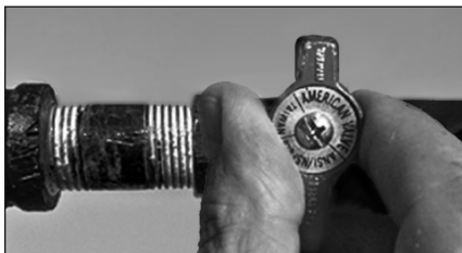
Figure 46 - Gas valve in "off" position.
