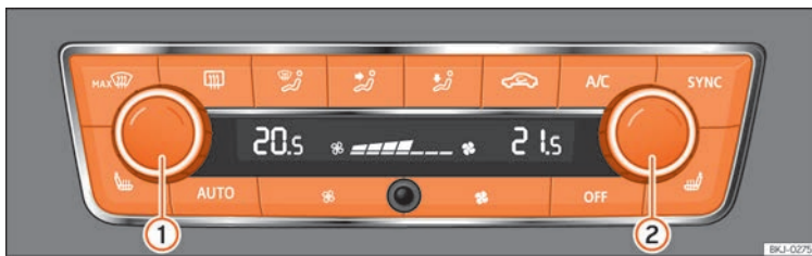
Fig. 82 In the centre console: Climatronic control panel.
