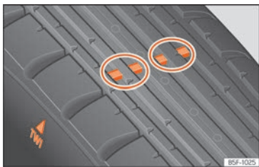
Fig. 181 Tyre profile: tread wear indicators.
