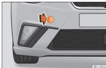
Fig. 155 Front bumper on right: remove the lid.
