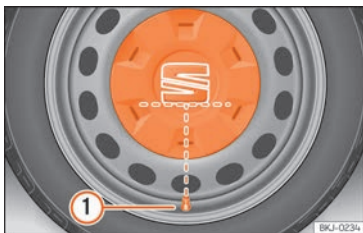
Fig. 184 Correct positioning of the central wheel trim for steel rims.
