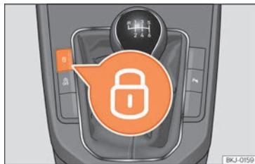
Fig. 53 Centre console: central locking switch.
