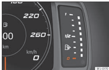
Fig. 6 SEAT Digital Cockpit instrument cluster: fuel gauge.
