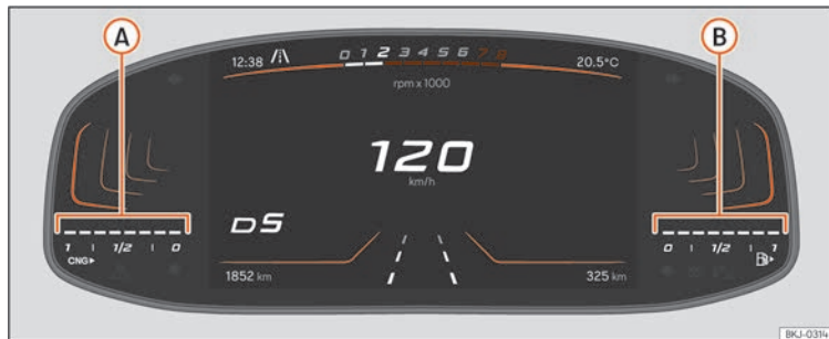
Fig. 7 Instrument cluster: natural gas gauge
