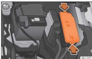
Fig. 160 In the engine compartment: lid of the fuse box.
