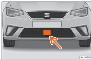
Fig. 96 On the front bumper: radar sensor.
