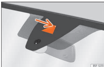
Fig. 98 On the windscreen: field of vision of the Lane Assist system camera.
