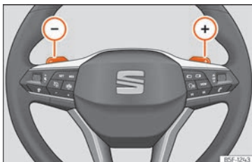
Fig. 91 Steering wheel: automatic gearbox levers
