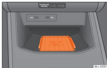
Fig. 135 Centre console: slot for mobile phone connection.
