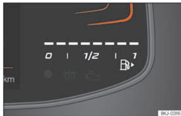
Fig. 5 Basic instrument cluster: fuel gauge.
