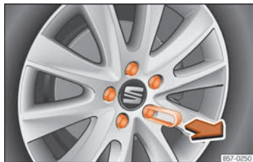
Fig. 186 Wheel: wheel bolts with caps.
