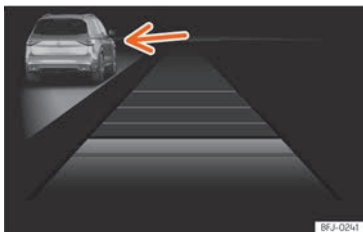
Fig. 106 On the instrument panel display: ACC active, vehicle detected on the left.
