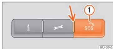
Fig. 45 On the roof console: controls for voice services
