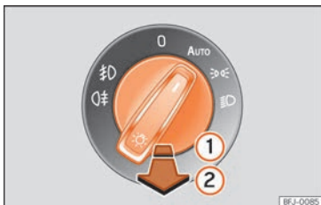
Fig. 73 Instrument panel: light panel.
