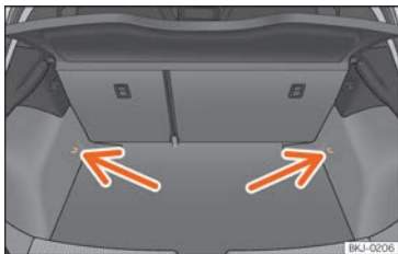
Fig. 140 Location of fastening rings in luggage compartment.
