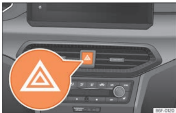
Fig. 44 Dashboard: switch for hazard warning lights.
