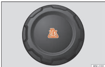
Fig. 172 Front compartment: coolant expansion tank cap.
