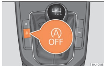
Fig. 87 Centre console: Start-Stop system button.
