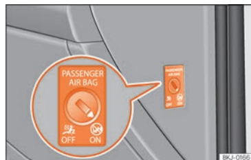
Fig. 30 Switch for activating and deactivating the front passenger airbag.
