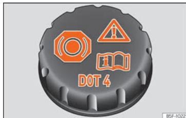
Fig. 173 Engine compartment: brake fluid reservoir cap.
