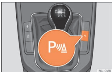
Fig. 120 Centre console: parking aid button (depending on the version).
