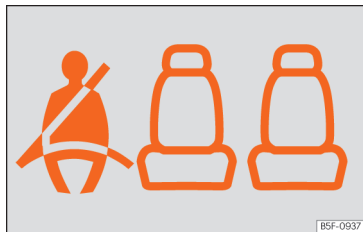
Fig. 21 Instrument cluster: indication of the status of the rear seat seat belts.
