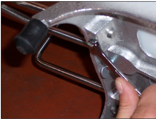
Figure 4. Pusher Head Adjustment Through the Blades.
