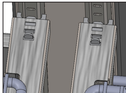
PROPERLY INSTALLED CLIPS
