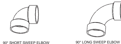
Figure 23. Vent Pipe Elbows
