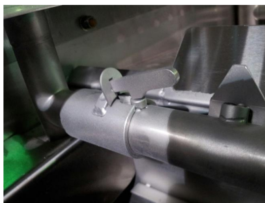
Rinse arm index notch, latch will drop as arm is pushed in
