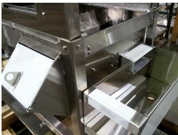
ADC-66 power scrapper, overflow to scrap box
