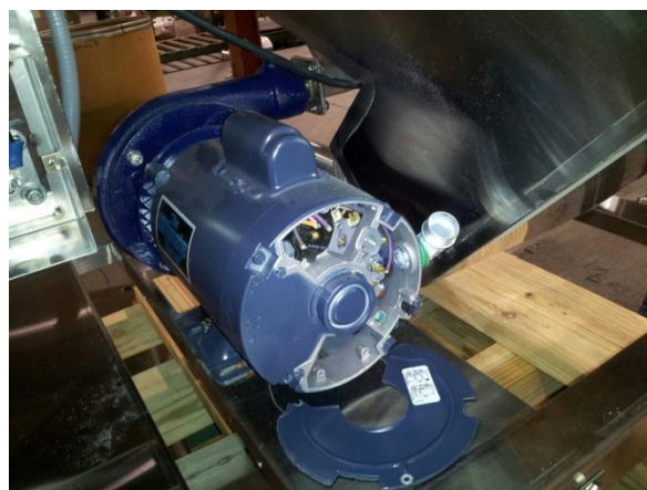
66 power scrapper motor, 1.5 HP, 208v, single-phase
