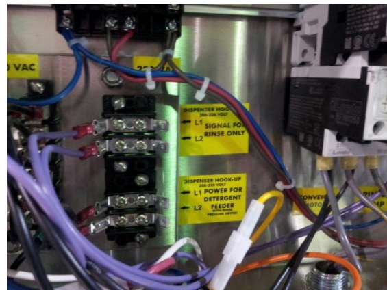
Dispenser signal connection terminals in control box
