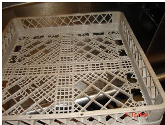
Damaged and broken rack that will jam or skip conveyor
