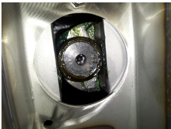
Cam bearing screws into cam block B
