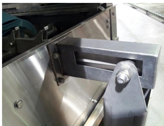
Rocker arm attached to conveyor bar, drip chute
