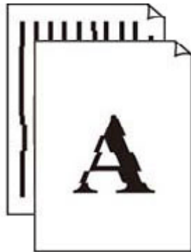
Lines Are Misaligned/Distorted
