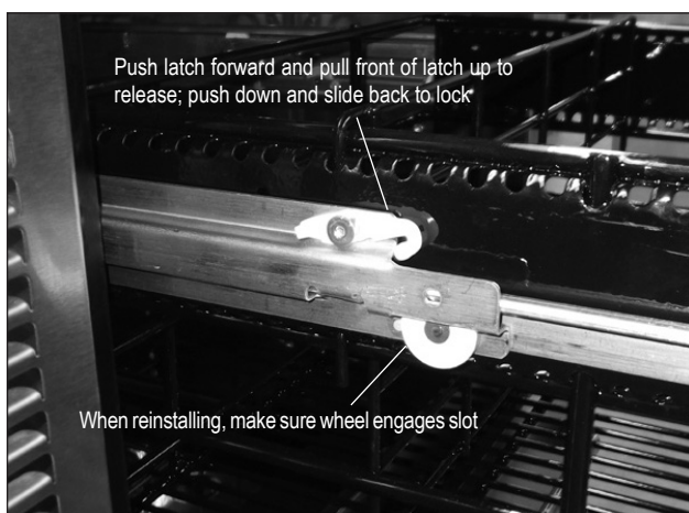
Figure 16: Removing/Installing Drawer
