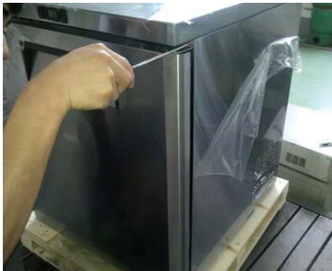
1) Unscrew the top hinge.
