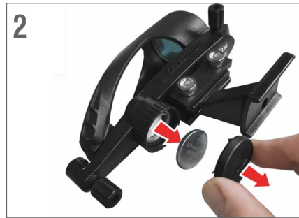
2. Remove the CR2032 battery from compartment.
