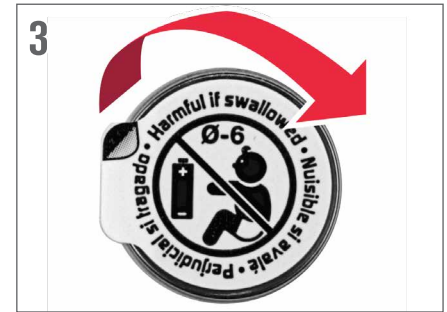
3. Peel off the sticker that is blocking the CR2032 battery's circuit.
