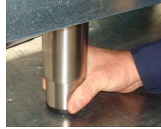
Adjust the legs to level the unit
