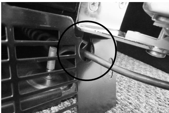
CORRECT Wire Position- Inside Grommet.
