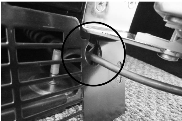
CORRECT wire position- Inside grommet.
