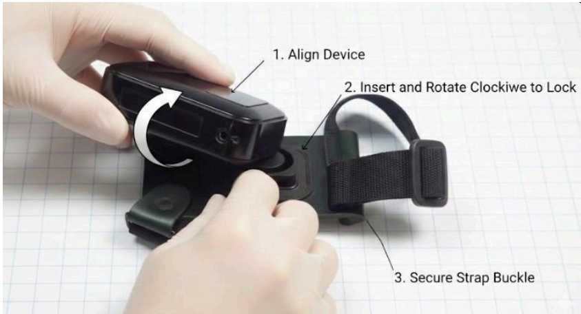
Figure 27. Connection between strap and connector
