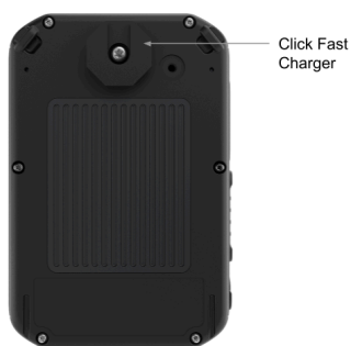
Figure 25. Klick Fast connector behind the device
