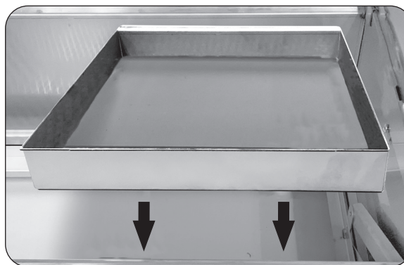
Fig. 12-2 Install charcoal pan(s)
