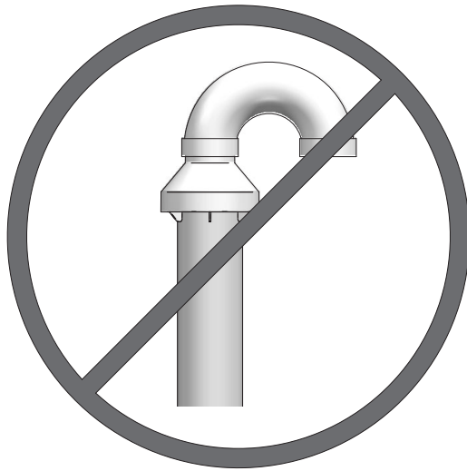
Figure 48. Do Not Install U-Bend to Rain Cap
