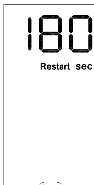
Compressor Protection Status
