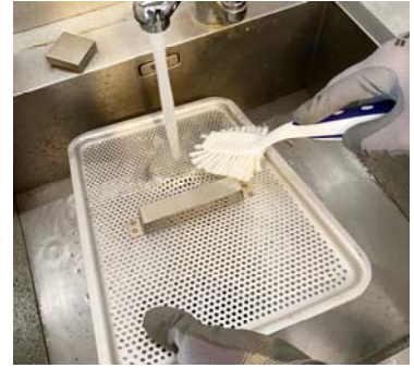
Clean the tank filter
