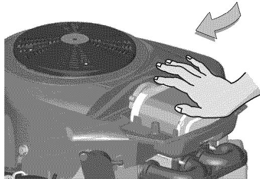
Figure 30. Air Filter Installation A. Filter Cartridge
