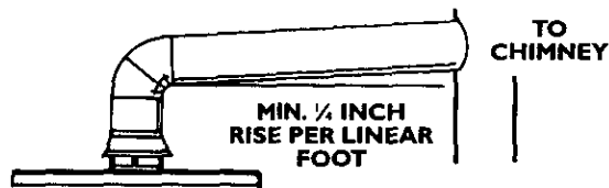
VENT PIPE INSTALLATION
