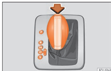
Fig. 235 Automatic gearbox selector lever with locking button (arrow)
