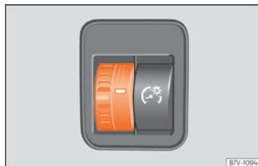
Fig. 119 Next to the steering wheel: instrument and switch lighting adjuster
