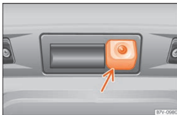
Fig. 246 In the rear bumper: location of the reverse assist camera.
