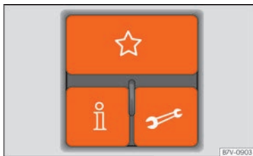
Fig. 85 Three button module in the roof: telephone management system controls.
