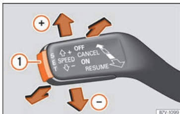
Fig. 248 On the left of the steering column: third lever for operating the GRA.
