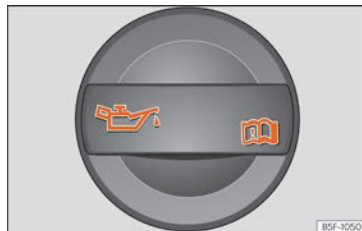
Fig. 288 In the engine compartment: Engine oil filler cap.
