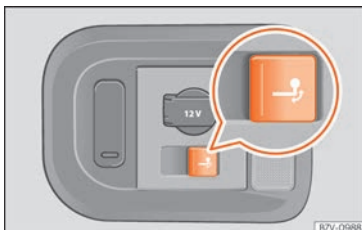
Fig. 276 On the right side of the luggage compartment: button for unlocking the tow hook.
