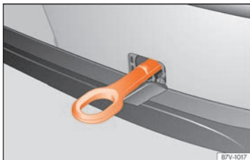
Fig. 57 On the right side of the rear bumper: towline anchorage in position.
