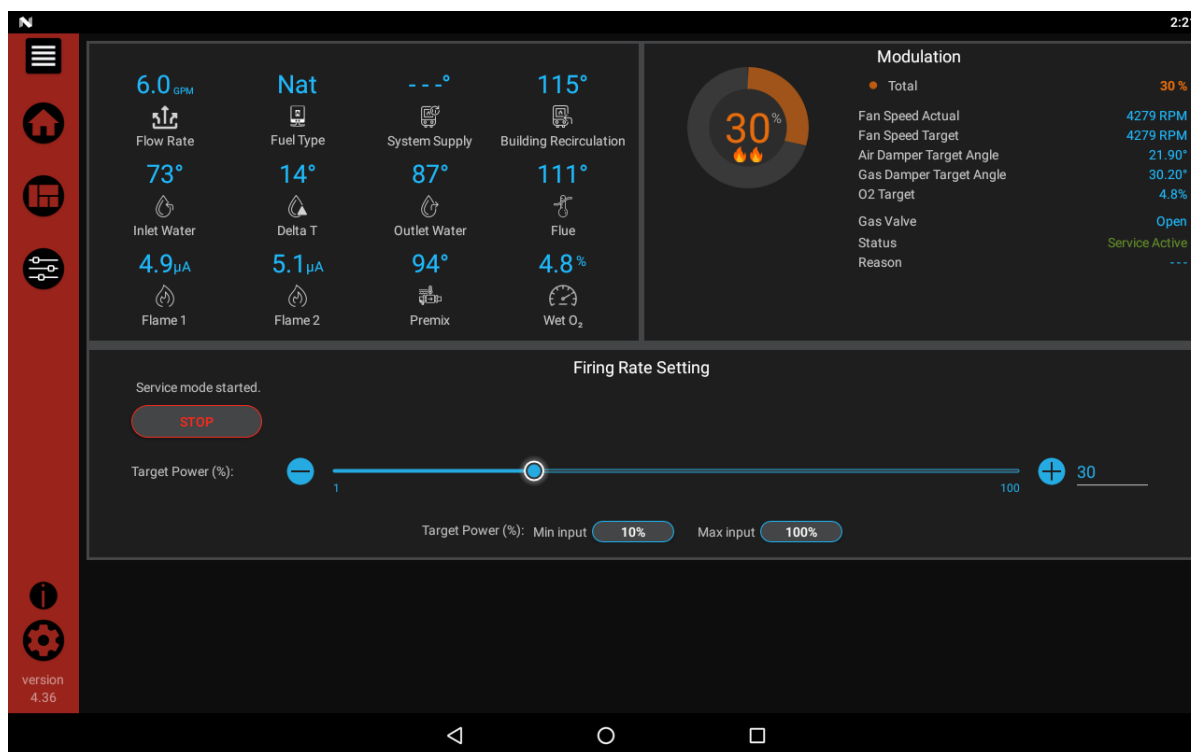
Figure 11-5 Service Maintenance Screen
