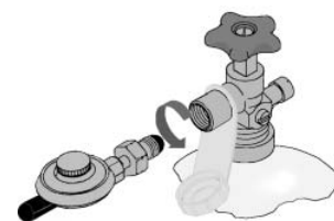
For POL cylinders, tighten counter-clockwise
