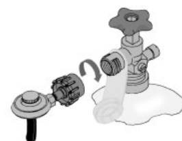
For Quick Connect cylinders, tighten clockwise
