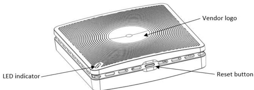
Figure 8 Base hardware characteristics (B700/730)
