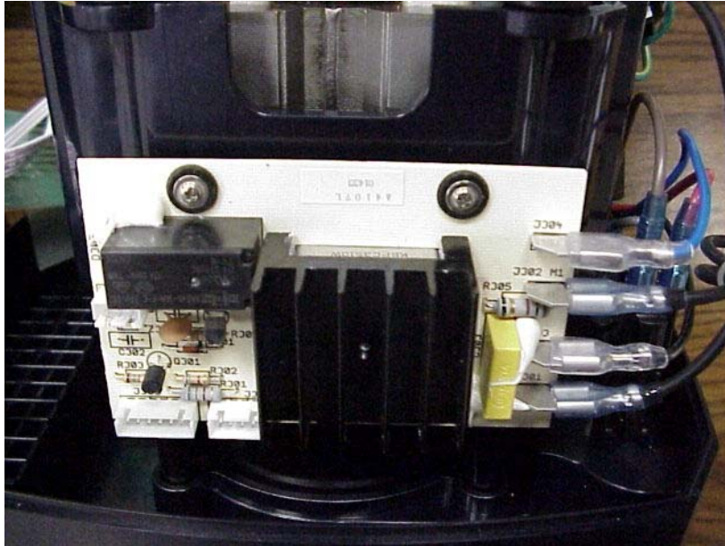
Figure 1. Power board Top Push on Connector is line voltage 1 leg (approx. 120V). Numbers 2, 3 and 4 are slightly lower reading; approx. 110V.
