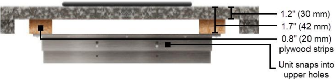
Figure 4-3: Stone Countertop 1.2" (30 mm) with Plywood Strips
