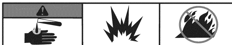
Battery acid is corrosive, explosive and flammable
