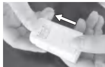
Figure 6: Along the direction of the arrow to open the battery cover
