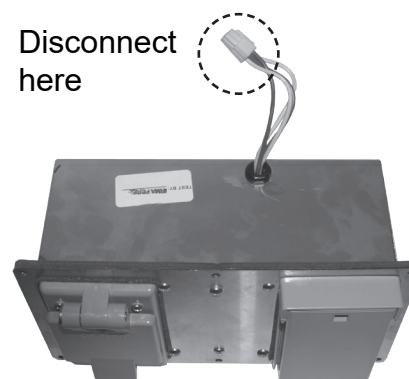
Fig. 49-2 Slightly pull out box and disconnect wire harness
