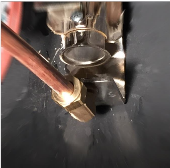
Fig 7.2 Nozzle-holder curve and damper sleeve
