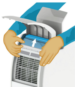
RETURN AIR INLET FILTER
