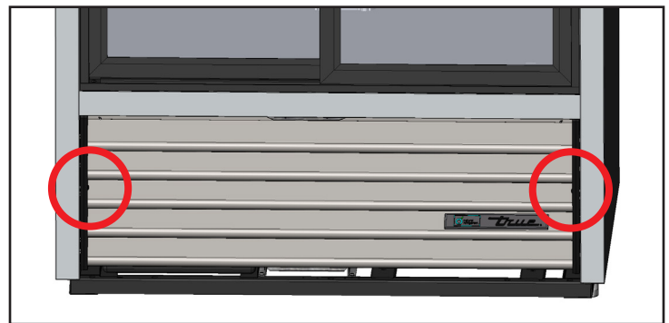
Fig. 2. Slide door louver grill screw locations.
