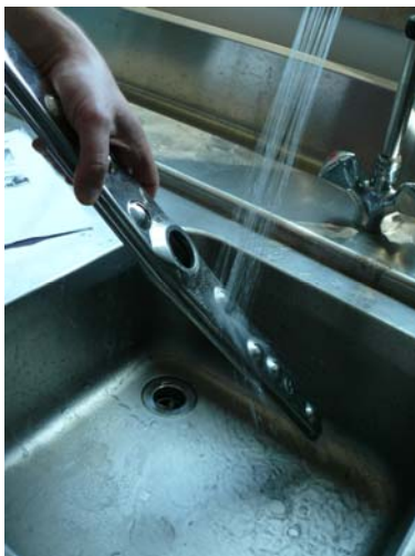
Clean the washing arm for any debris inside.
