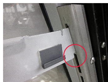
Top notch installed (gap)
