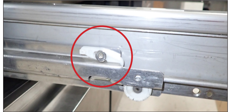
Fig. 1. Drawer retainer location. Retainer is engaged.
