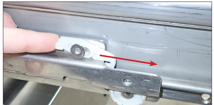
Fig. 2a. Push the retainer forward.
