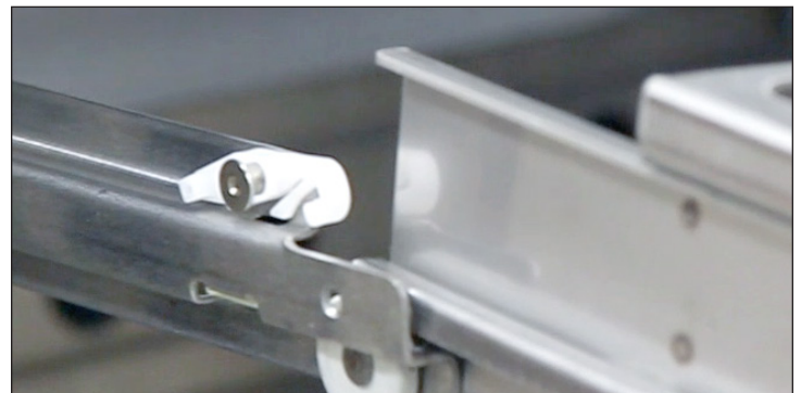
Fig. 3. Align the drawer with the drawer slide.
