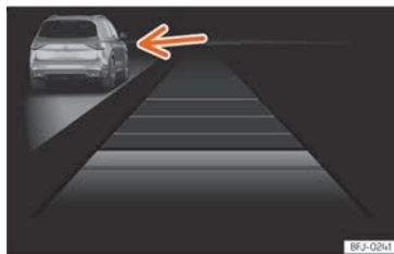
Fig. 132 On the instrument panel display: ACC active, vehicle detected on the left.
