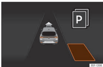
Fig. 150 On the instrument panel display: display of the assisted parking system with decreased visibility.
