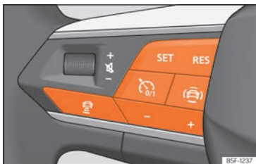
Fig. 131 On the multifunction steering wheel: buttons for operating the ACC.
