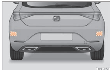
Fig. 125 Rear view of the vehicle: radar sensor areas.
