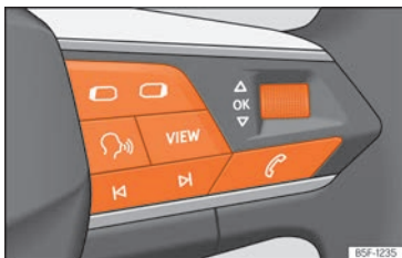
Fig. 15 Right side of multifunction steering wheel: buttons to the menus and informative indications on the instrument panel (depending on the version).
