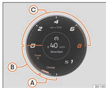
Fig. 11 Digital instrument cluster: Power meter
