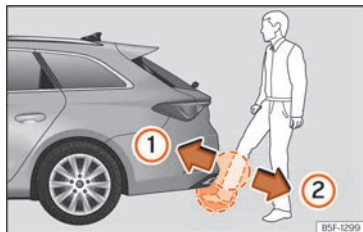
Fig. 81 Rear lid with sensor-controlled opening (Easy Open).
