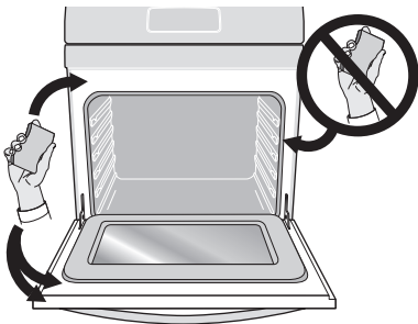
Figure 21: Clean around the oven door gasket
