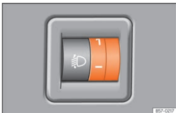
Fig. 73 Next to the steering wheel: regulator headlight range control.
