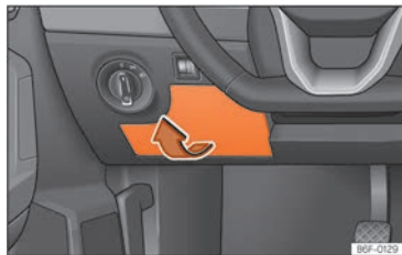
Fig. 167 On the dashboard on the driver side: lid of the fuse box.
