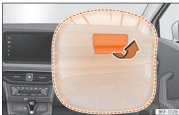
Fig. 29 Front passenger airbag located in dash panel.
