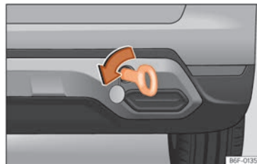
Fig. 166 Right side of the rear bumper: towline anchorage screwed in.
