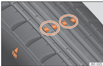
Fig. 189 Tyre profile: tread wear indicators.
