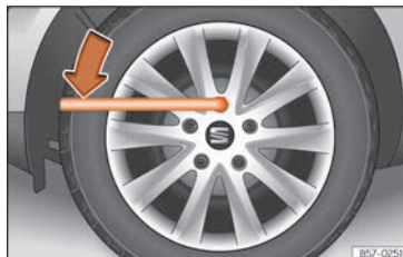
Fig. 195 Tyre change: slacken the wheel bolts.
