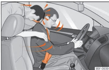
Fig. 23 Any rear seat occupants not wearing a seat belt may be thrown forward violently, hitting the driver who is wearing the seat belt.
