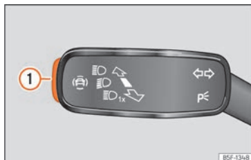
Fig. 92 On the turn light and main beam lever: key for driver assistance systems (depending on the version).
