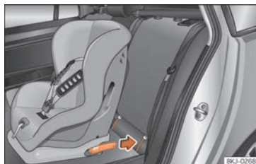
Fig. 39 Rear seats: fitting a child seat with the ISOFIX system.
