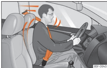
Fig. 20 Drivers with properly worn seat belts will not be thrown forward in the event of sudden braking.
