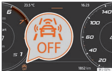
Fig. 109 On the screen of the instrument panel Front Assist switched off message.
