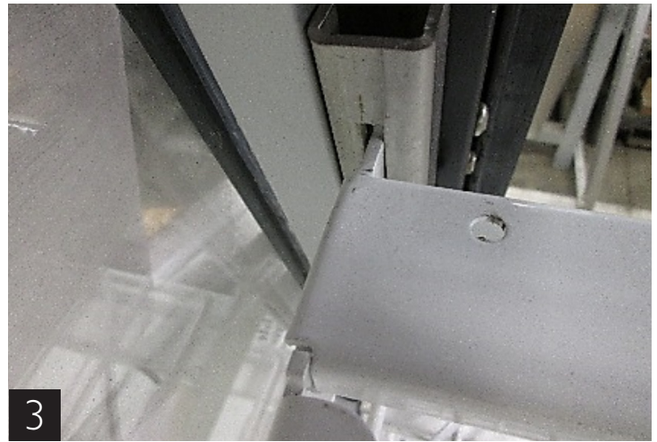
Light assembly installed on shelf support
