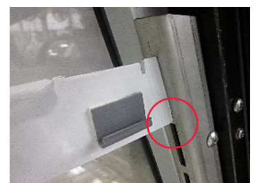
Bottom notch installed (no gap)
