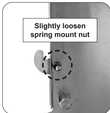
Fig. 41-3 Slightly loosen nut
