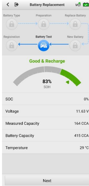
Figure 6-2 Sample New Battery Test Results Screen
