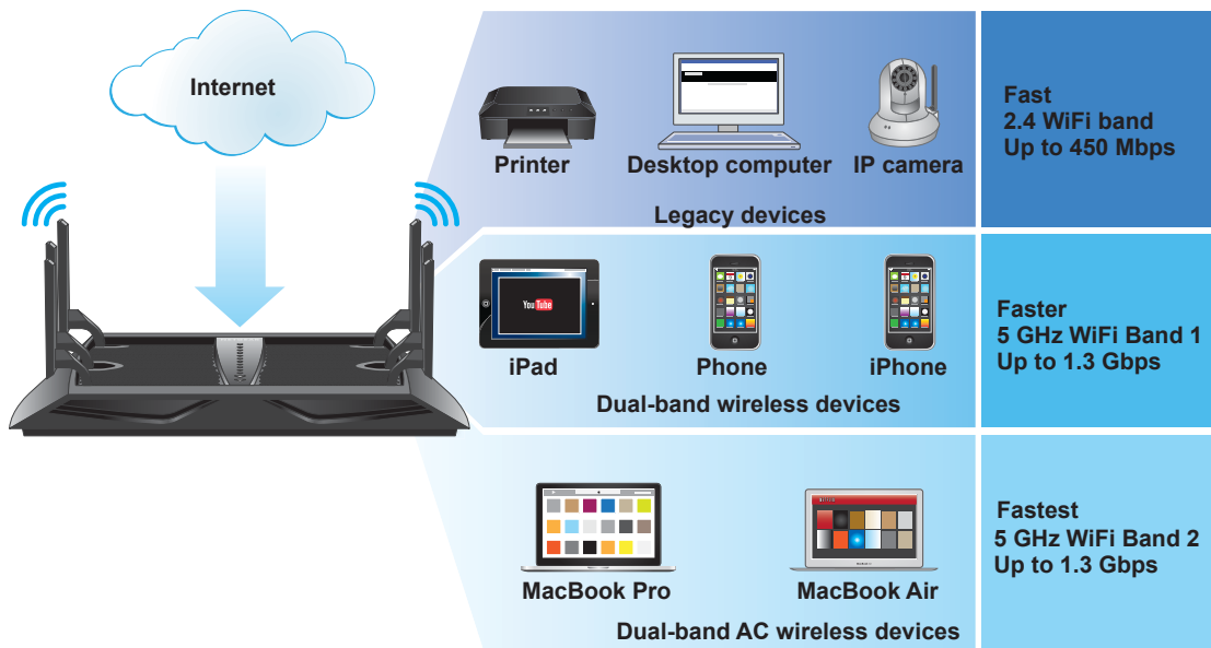
Figure 10. Load balancing in a tri-band WiFi network
