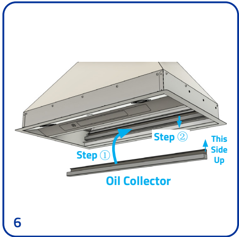
Set the oil collector to the correct position and place it into the rear slot.
