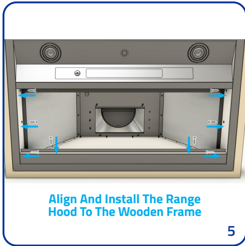
Align and install the range hood to the wooden frame.
