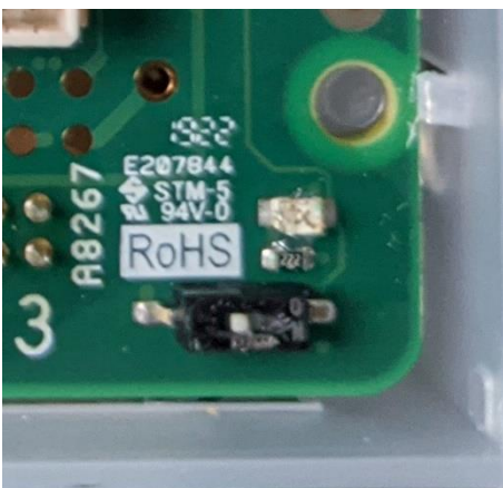
Figure 16 – Correct switch position
