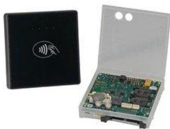
Figure 1 – KarL4 contactless terminal
