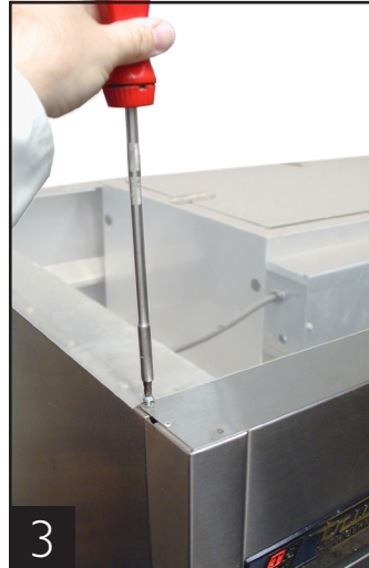
Rainshield removal, top screws.
