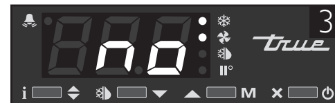
Image 3: If "no" appears on screen, the controller is unlocked.
