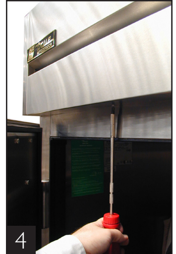
Rainshield removal, bottom screws.
