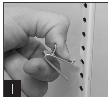
1 Installing top tab of shelf clip
