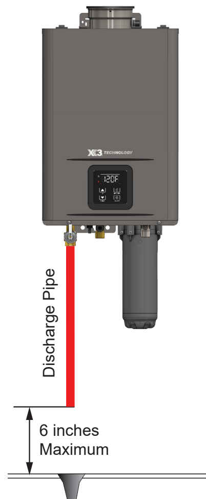
Figure 21 - Discharge Pipe Clearance
