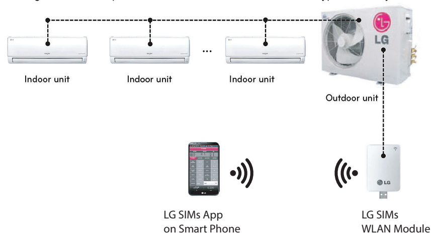
Figure 135: Example of a SIMS WLAN Module Used with a Typical DFS System.
