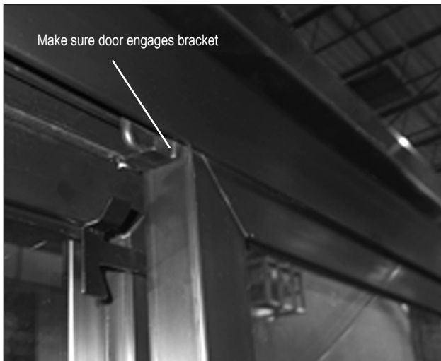
Figure 14: Removing/Installing Sliding Door
