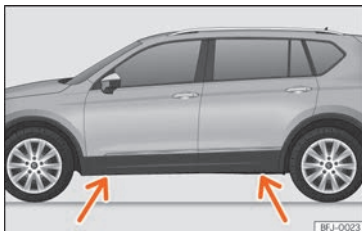
Fig. 254 Jack position points.
