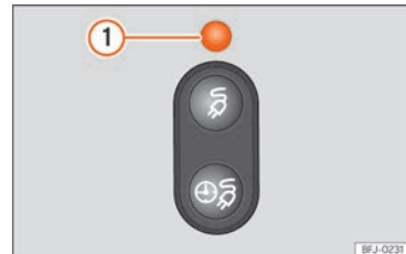
Fig. 56 Behind the battery charging socket cover: charging process indicator.
