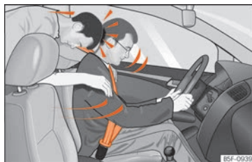
Fig. 24 Any rear seat occupants not wearing a seat belt may be thrown forward violently, hitting the driver who is wearing the seat belt.
