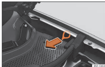
Fig. 58 Between the left wing panel and the engine bonnet hinge: Charging connector manual release mechanism puller.
