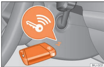
Fig. 119 On the right of the steering column: emergency start.
