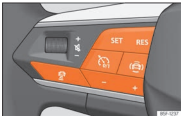
Fig. 140 On the multifunction steering wheel: buttons for operating the ACC.
