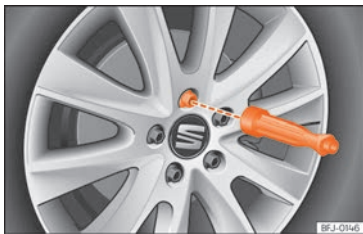
Fig. 256 Changing the wheel: unscrew wheel bolts with the socket at the end of the wheel brace.
