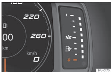
Fig. 7 SEAT Digital Cockpit instrument cluster: fuel gauge.
