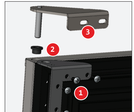
Fig. 7b. Top hinge component assembly.
